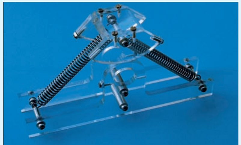
Demonstration model with two springs acting on the same point of the moving part, which is in a state of equilibrium in any position. The springs counterbalance each other.
