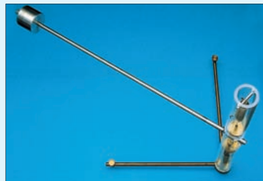
Demonstration model of an indifferent equilibrium. The weighted rod will remain stable in any position. The dynamically equivalent resultant of the two springs acts on the centre of gravity of the mass. This is an example of a floating hinge.
