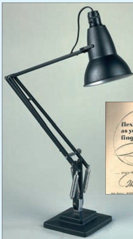
Anglepoise desk lamp with special springs. It is exactly balanced and will retain any attitude it is given, even if there were no friction in the hinges.
