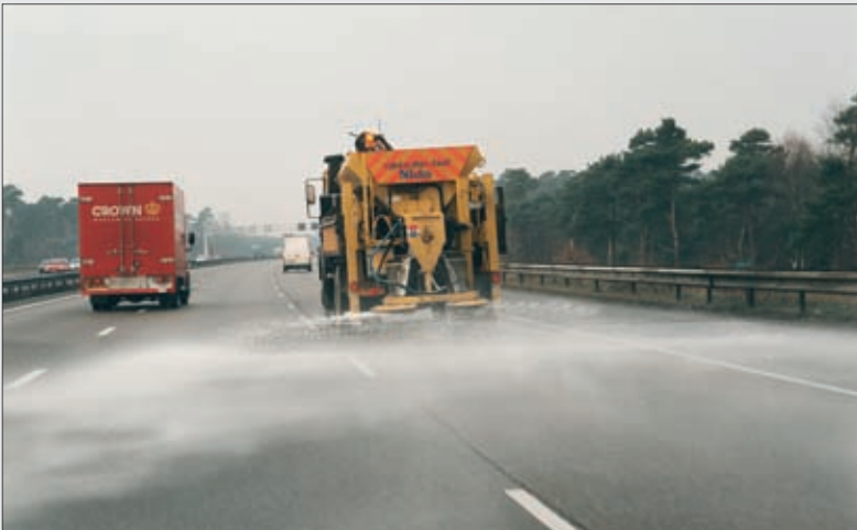
Many salts used for de-icing are chlorides that in the long term will cause corrosion in concrete structures.
