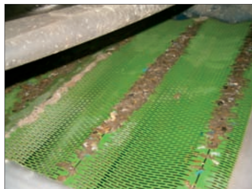
Spanwelle- lter, with a continuously reforming flexible lter screen, which prevents clogging.
