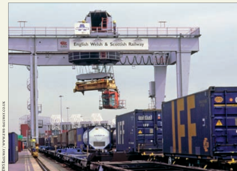
The gantry cranes are fitted with a spreader that can be rotated so containers will always be loaded onto the train with the door ends facing each other. One of the reasons this is done is to prevent theft.
